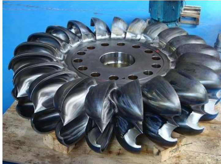
Gambar 2.3 Runner Turbin Pelton
