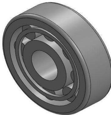
Gambar 4.11 Hasil Rancangan Bantalan Bearing
