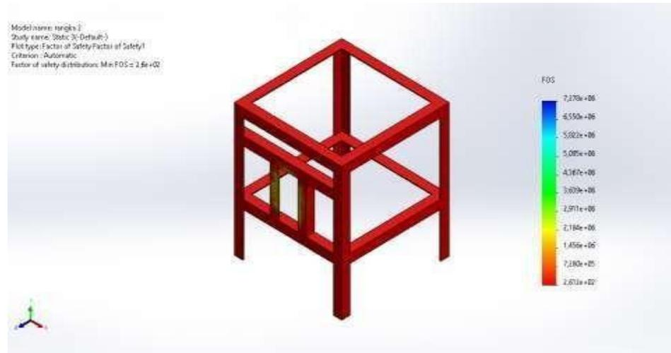
Gambar 4.21 Hasil Pembebanan *factor of safety*
