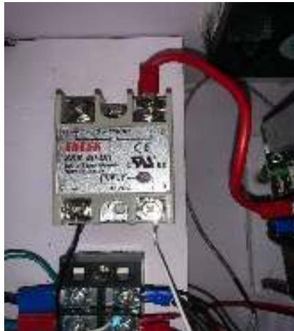
Gambar 3. 12 SSR ( Solid State Relay)
