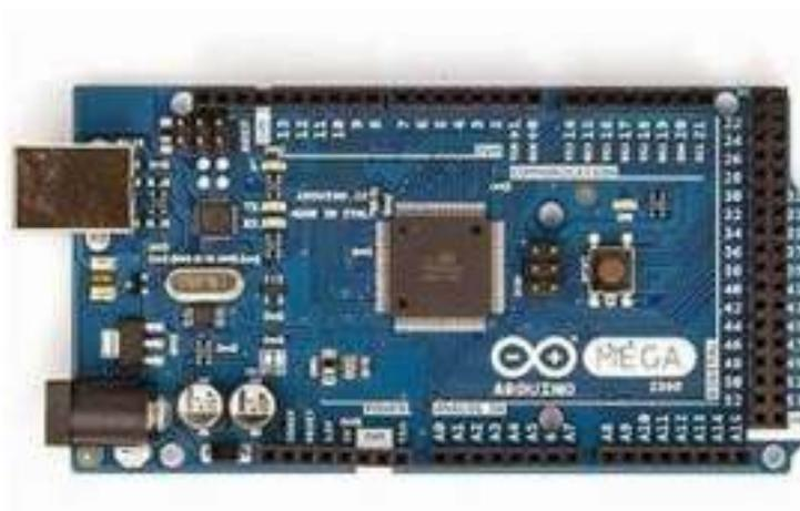
Gambar 2. 8 Arduino Mega 2560 (Arduino dan Sensor Pada Project Arduino DIY, n.d.)
