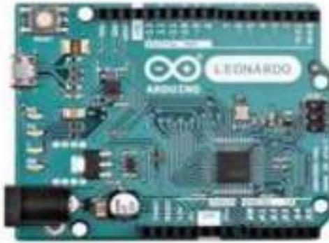
Gambar 2. 6 Arduino Leonardo (Arduino dan Sensor Pada Project Arduino DIY, n.d.)
