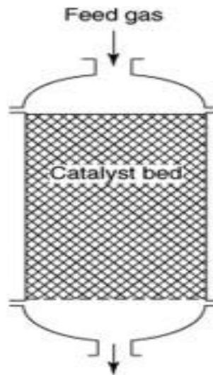
Gambar 2.9 *Adiabatic fixed-bed reactor* (Eigenberger, 1972)
