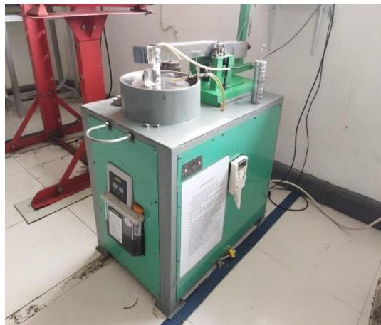
Gambar 3.2 Mesin Tribometer pin on disc
