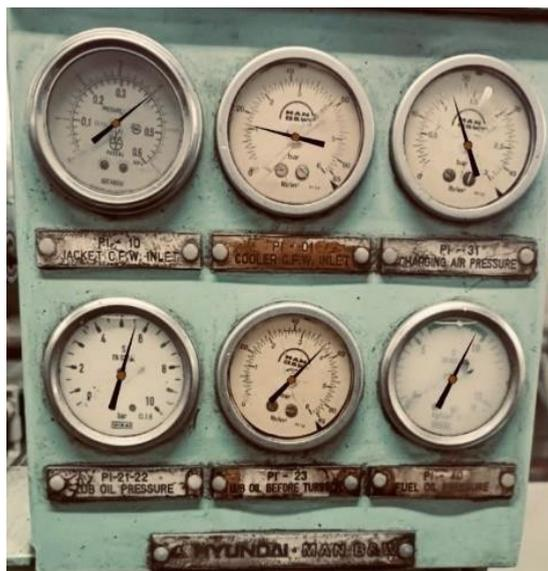
Gambar 4.1 Panel Indikator Tekanan Diesel Generator
