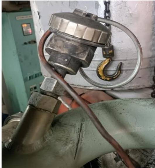
Gambar 3.3 *Thermocouple*
