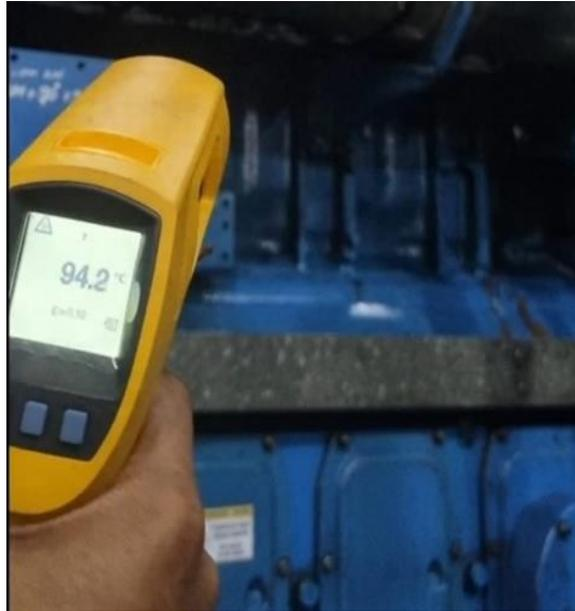
Gambar 4.6 Suhu *Cylinder Head* Yang Melebihi Batas Normal
