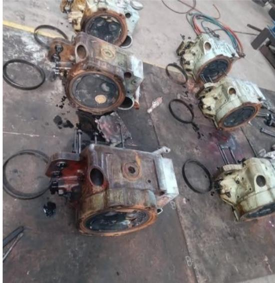
Gambar 4.7 *Cleaning Cylinder Head*
