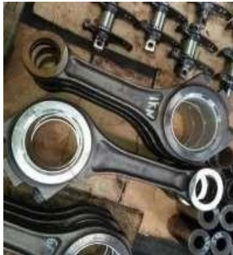
Gambar 2.7 *Connecting Rod* (Priambodo, 2020).
