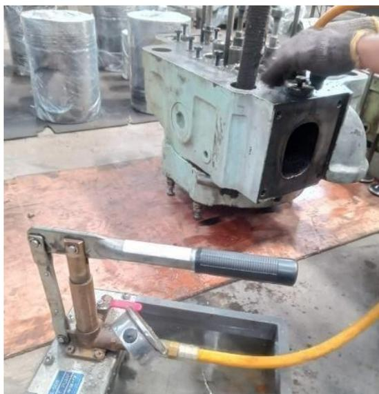
Gambar 4.8 Tes Kebocoran *Cylinder Head*
