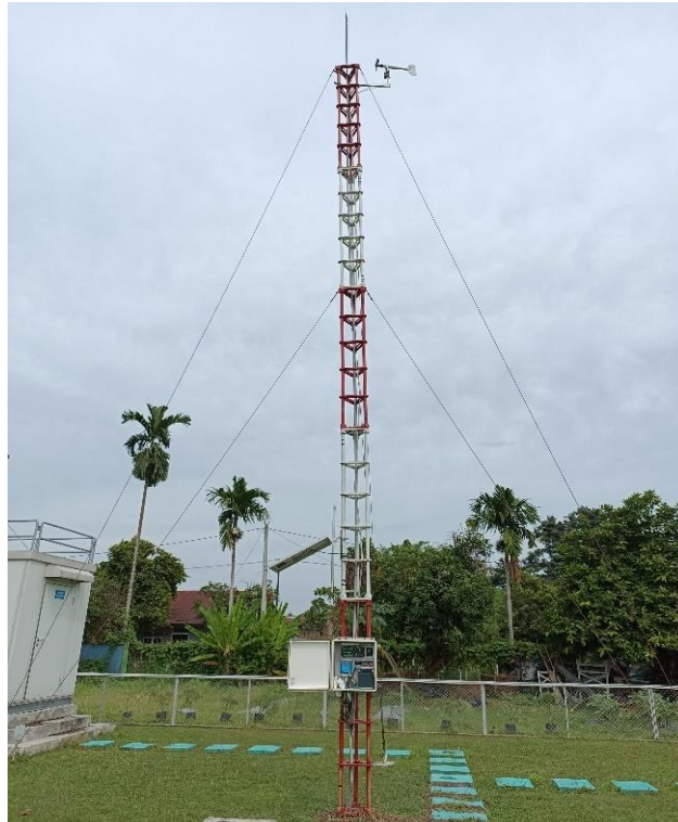
Gambar 4.14. Automatic Weather Station
