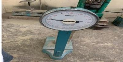
Gambar.4.10.Penimbangan Sampel Beton Tulangan Besi
