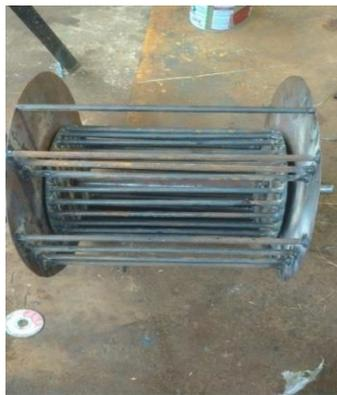
Gambar 4.4 Ripple Mill
