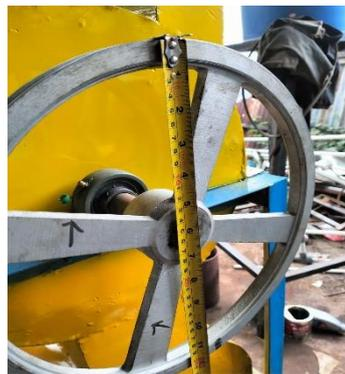
Gambar 4.2 Pulley Ripple Mill
