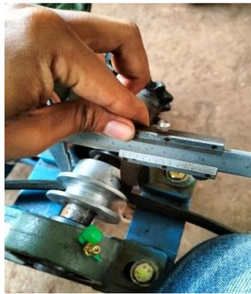
Gambar 4.15 Pulley Output Gearbox
