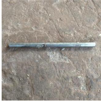
Gambar 4.3 Poros Ripple Mill
