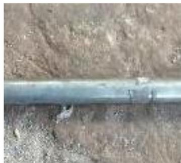
Gambar 4.16 Poros Output Gearbox
