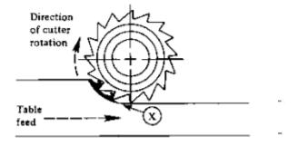
Gambar 2.6 *Conventional Milling* (Arian Metal)
