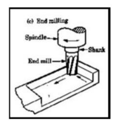
Gambar 2.5 End Milling (Researchgate)
