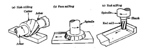
Gambar 2 .2 Dasar operasi milling (a) slab milling, (b) face milling, (c) end milling (Hestanto)
