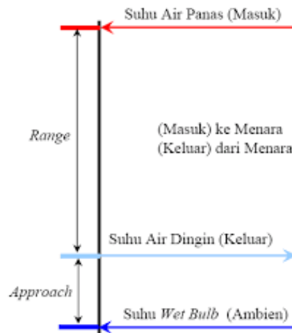
Gambar 2.6 Range & Approach Temperatur Cooling Tower (Handoyo, 2015)
