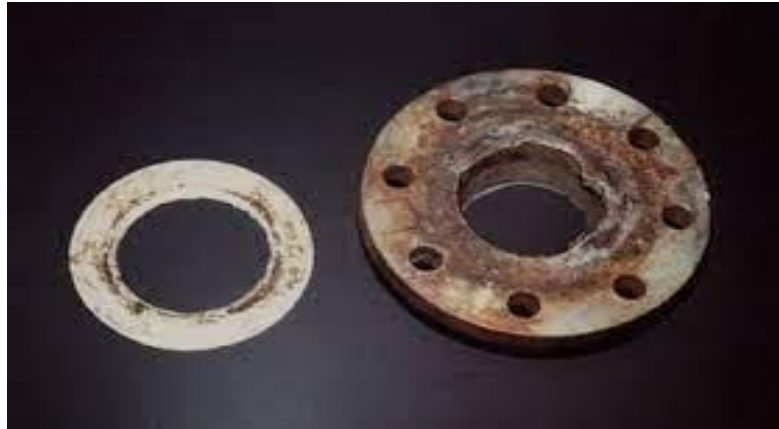
Gambar 2.6 Korosi Celah (Crevice Corrosion)
