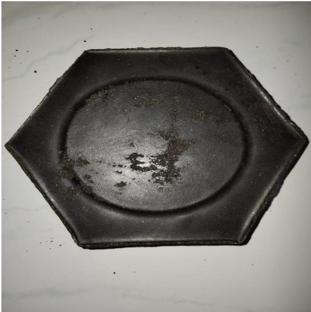
Gambar 4.22 *Paving Block* komposisi 40% : 60%
