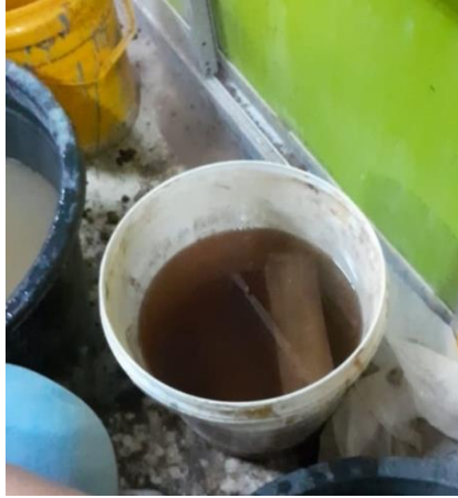
Gambar 4.9: Proses perendaman bata didalam air
