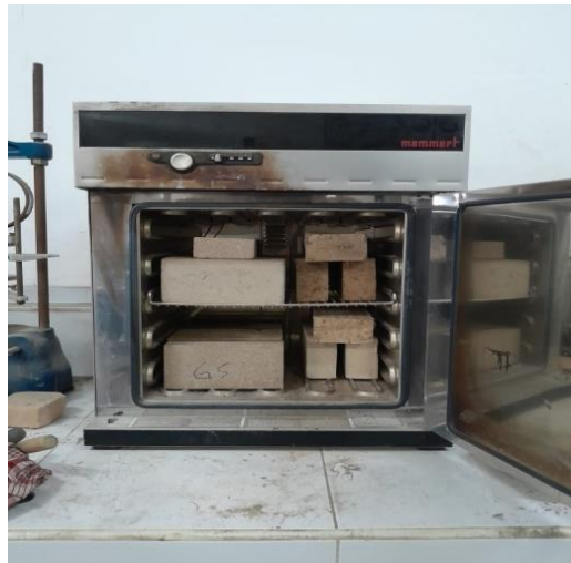
Gambar 4.8: Proses pengeringan bata didalam oven
