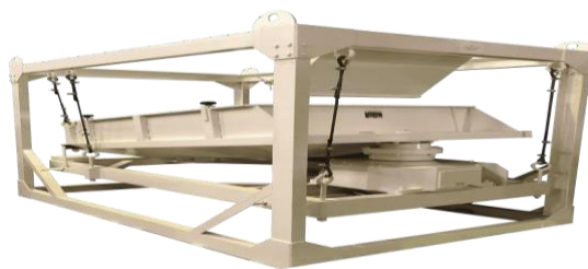
Gambar 2.4 Ayakan Reciprocating Screen (Handra et al., 2019)
