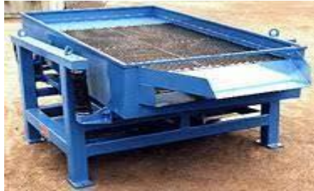
Gambar 2.5 Ayakan Shifting Screen(Ramadhansyah, 2021)
