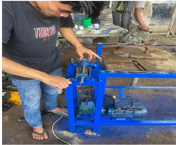
Gambar 4.31 Pemasangan bantalan ucp dan as
