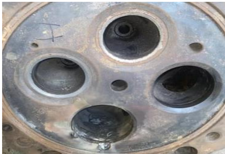
Gambar 4.14 Hasil pengelasan Cylinder Head
