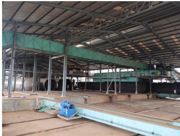
Gambar 2. 2 Real track Transfer carriage
