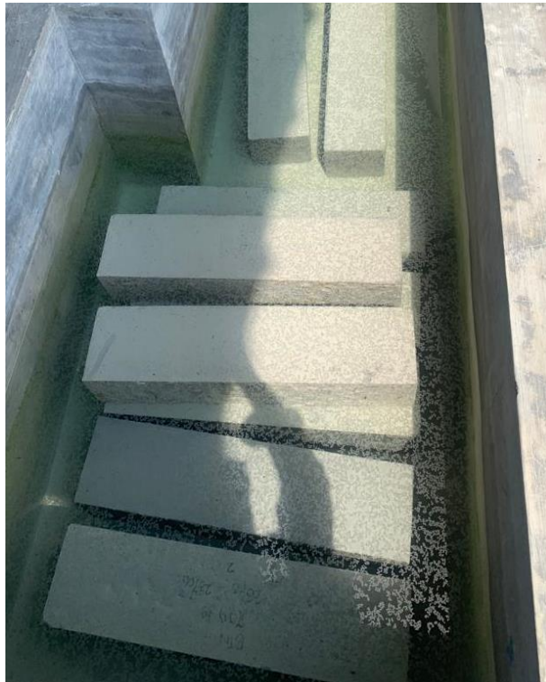
Gambar L.16 : Perendaman (Curing) Beton Balok
