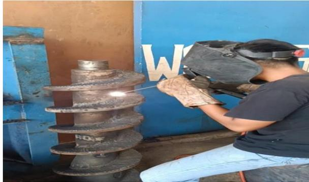
Gambar 4.4 *Rebuild Screw Press Tahap Pertama*
