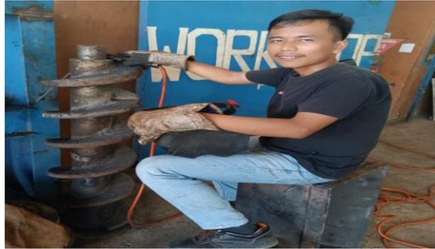
Gambar 4.5 *Rebuild Screw Press* Tahap Pertama
