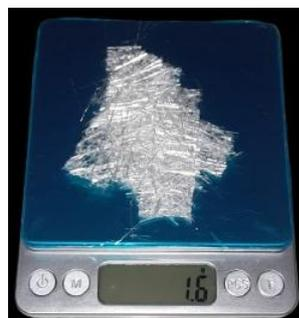
Gambar 4.6 Potongan fiber glass.
