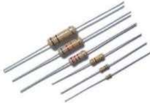
Gambar 2.23 Resistor Arang ( Carbon Resistor )
