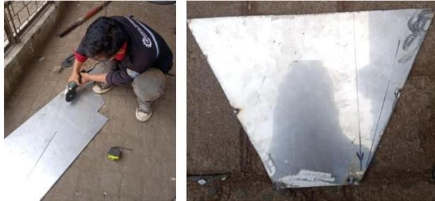
Gambar 4.43 Proses Pemotongan Dinding Hopper
