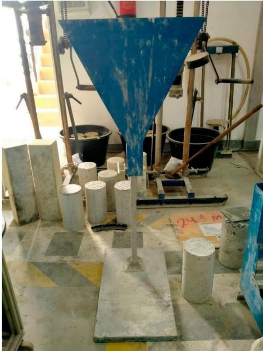
Gambar L.3: Alat pengujian V funnel
