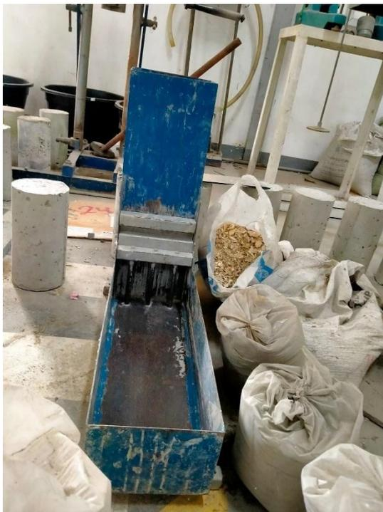
Gambar L.4: Alat pengujian L-Box
