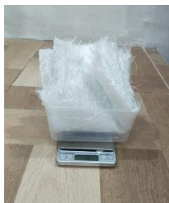
Gambar 4.3 Menimbang Fiber Glass
