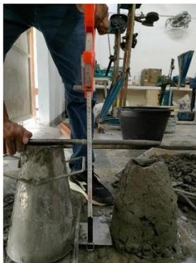
Gambar L. 3 Uji Slump Test
