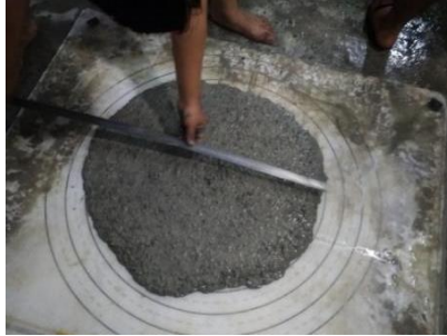
Gambar 3.4: Pengukuran diameter slump flow beton segar
