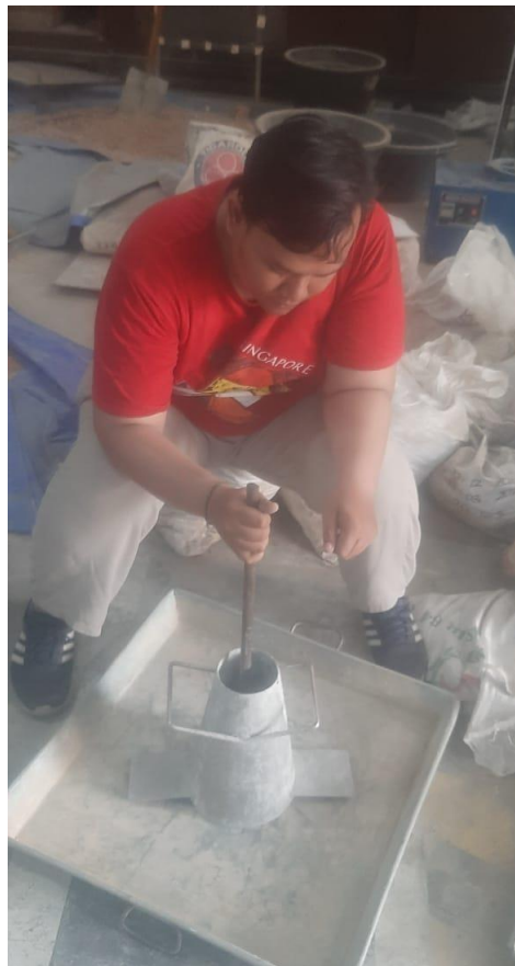
Gambar L6: Proses Uji Slump Test
