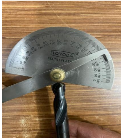
Gambar 4.4 proses mengukur sudut twist drill
