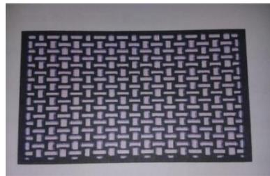
Gambar 2. 4 Woven Fiber Composite (bi-directional)
