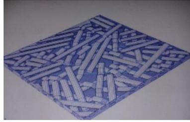
Gambar 2. 5 Hybrid Fiber Composite
