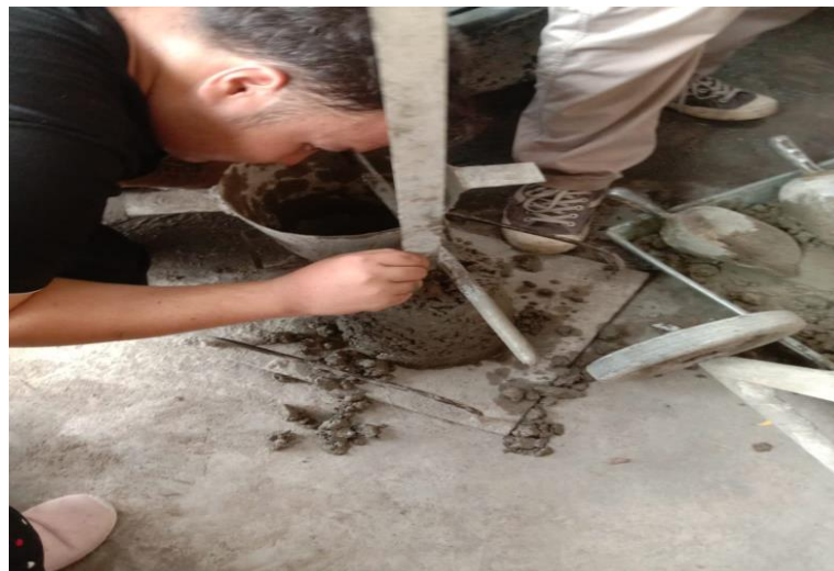
Gambar 3.9 Slump Test benda uji
