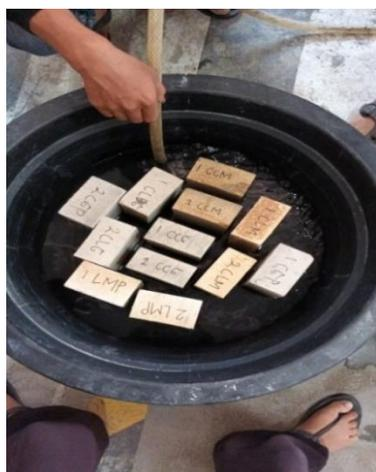
Gambar L-20 Uji Kadar Garam
