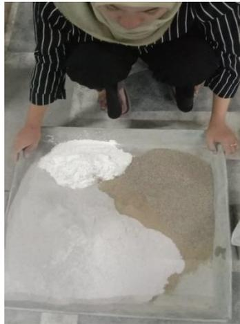
Gambar L-17 Bata Variasi Campuran Kapur + Tanah Galong + Pasir + ASP
