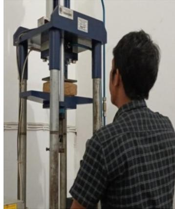
Gambar L-14 Alat Uji Kuat Tekan (Compression Test)
