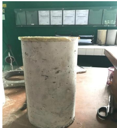
Gambar L- 8: Proses Capping Benda Uji
