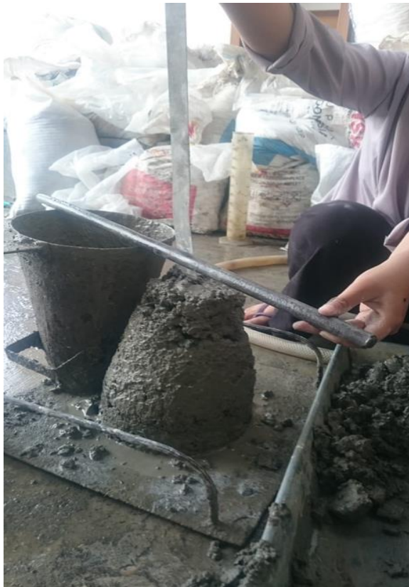
Gambar L.5: Pengujian slump test
