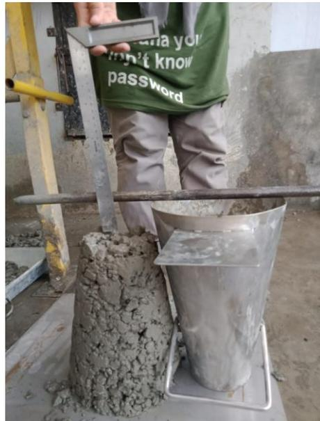
Lampiran 4 Uji Slump Test
