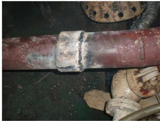
Gambar 2.5 korosi galvanis (Treathevey, 1991)
