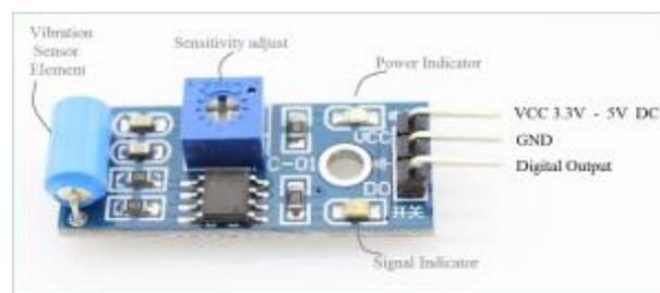
Gambar 2.13. *Vibration Sensor SW-420*
