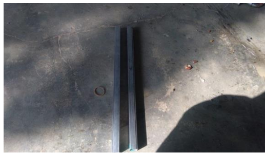
Gambar 4.55. Hasil Peemotongan Hollow Stainless Steel
