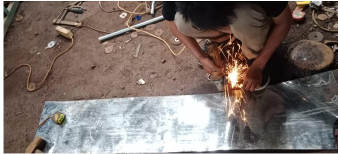
Gambar 4.5. Memotong Plat Stainless Steel
