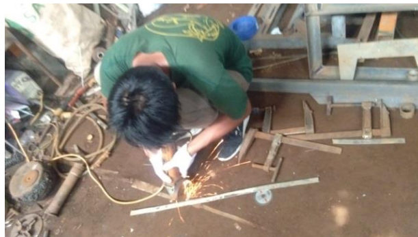
Gambar 4.47 Proses Pemotongan Plat Strip Stainless Steel
