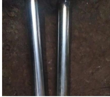
Gambar 4.17. Hasil Pemotongan Pipa Stainless Steel
