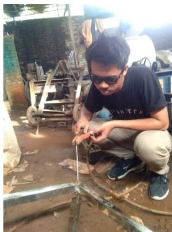
Gambar 4.41. Proses Pengelasan Hollow Stainless Steel
