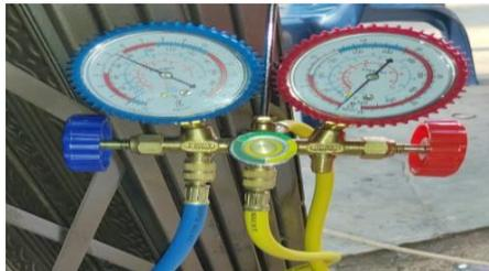
Gambar 3.14 Manifold Gauge
