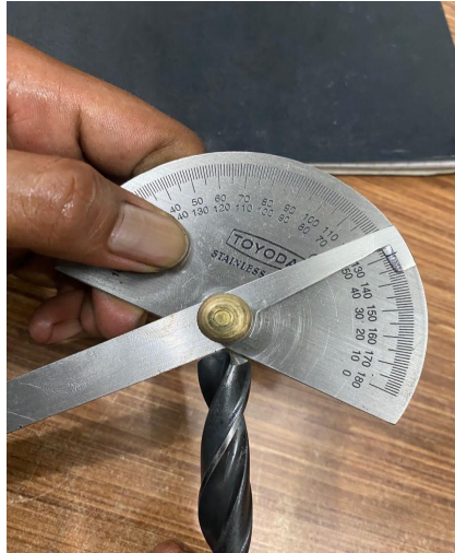
Gambar 4.3 proses mengukur sudut twist drill
