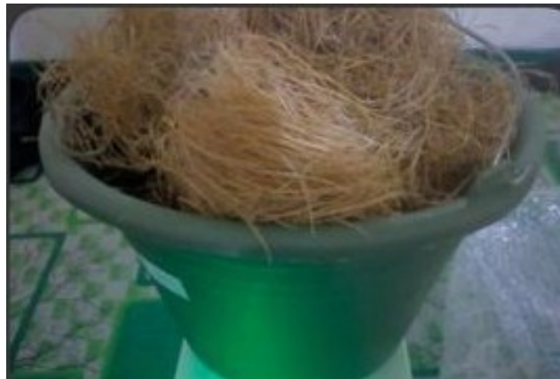
Gambar 3.17 Proses perendaman bahan kimia selama 1, 3, 5, 7, 9 jam
