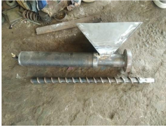
Gambar 3.32 Hasil perancangan screw
