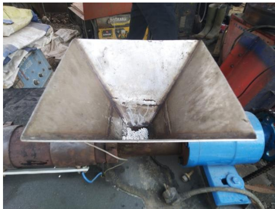
Gambar 3.35 Proses Pengujian Mesin Extruder plastic
