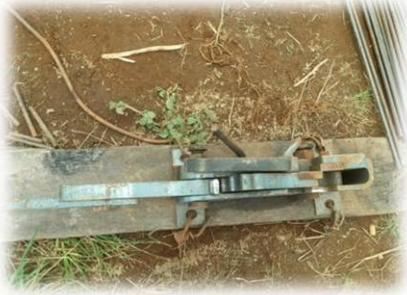
A manual steel rebar cutter, also known as a rebar bender, lying on a concrete surface. It has a long handle and a cutting mechanism. | Pemotong baja tulangan       |
