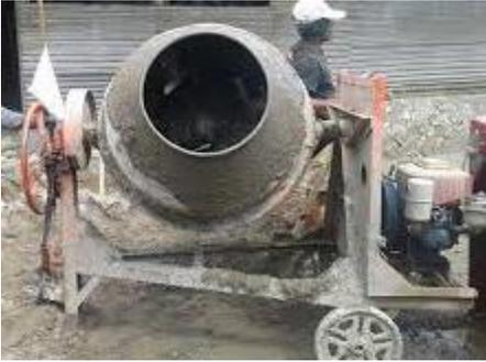
A concrete mixer machine with a large rotating drum, mounted on a metal frame with a wheel, powered by a small engine. | Mesin Molen      |
