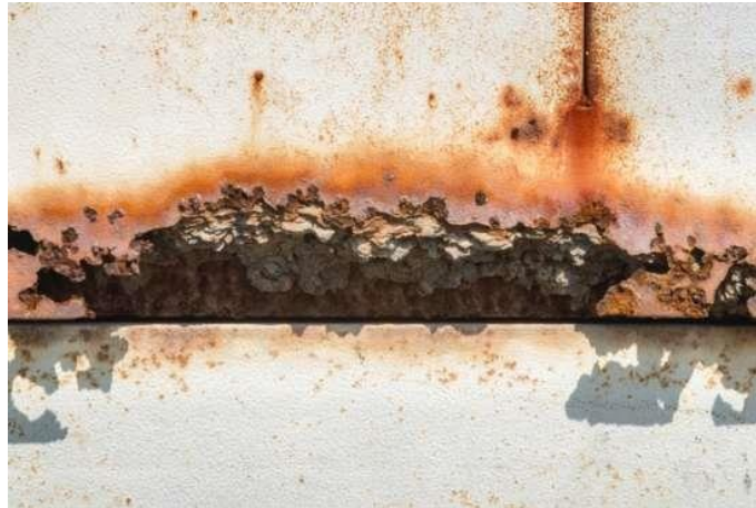
Gambar 2.2 Pitting Corrosion (Korosi Sumur) (C. Merola, 2017)
