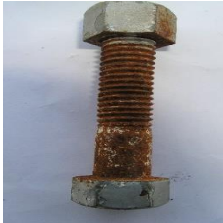
Gambar 2.6 Crevice corrosion ( korosi celah ) (Wibowo, 2012)
