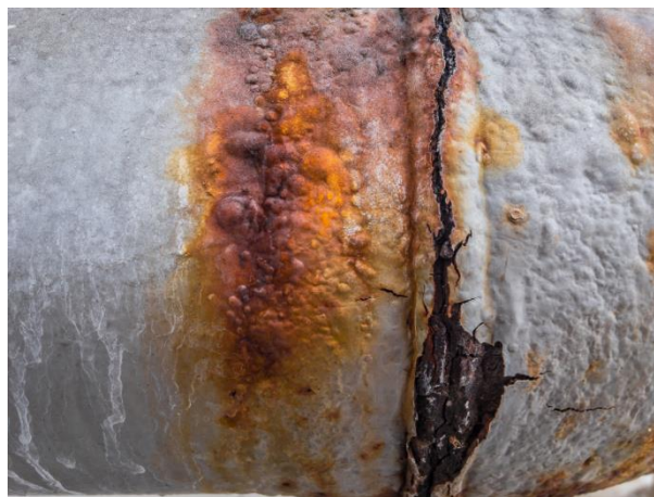
Gambar 2.5 Stress Corrosion (Korosi Tegangan) (Finchen Parsons, 2020)
