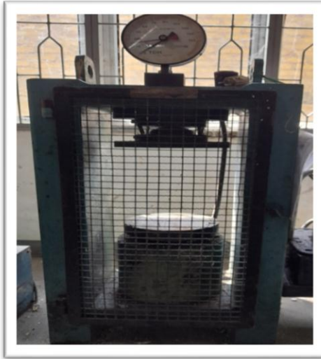
Gambar 3.19: Compression Machine Test.
