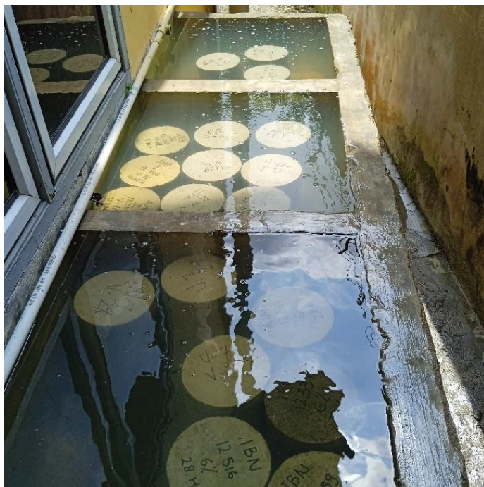
Proses perendaman beton
