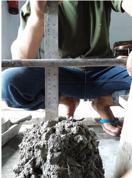
Proses pengujian Slump
