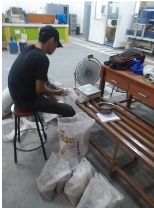
Proses penimbangan agregat
