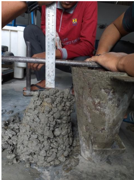
Lampiran 27 : Proses Pengujian Slump Test
