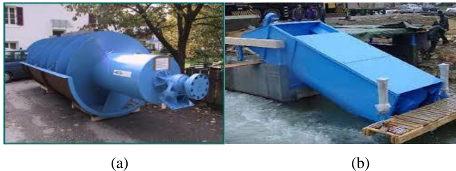
Gambar 2.2 Turbin Screw (a) Tipe Steel Strough dan (b) Tipe Closed Compact Installation (Lius, 2009)
