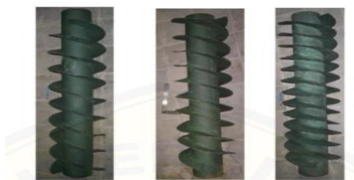
Gambar 1.1 Tiga Macam Model Turbin Ulir (Hizhar et al., 2017)
