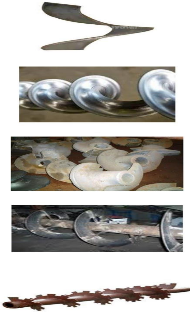
Gambar 2.13 Sectional Screw, Helicoid Screw, Cast Iron, Riboon, Cut Flight (Istiqlaliyah, 2013)
