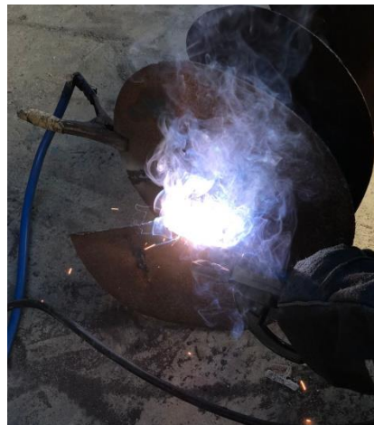
Gambar 4.18 Pengelasan Bagian Depan Screw.
