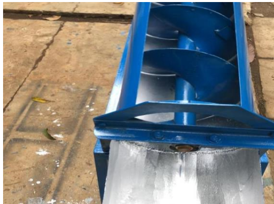
Gamabar 4.45 Pengecatan Turbin Screw.
