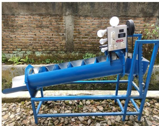
Gambar 2.1 Turbin Archimedes Screw
