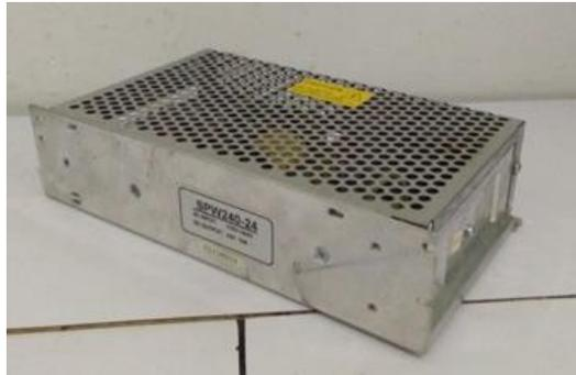
Gambar 3. 13 *Power Supply 20V 10A*
