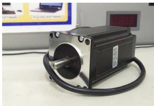
Gambar 3. 9 *Motor Stepper Nema 23 Torsi 3 Nm*
