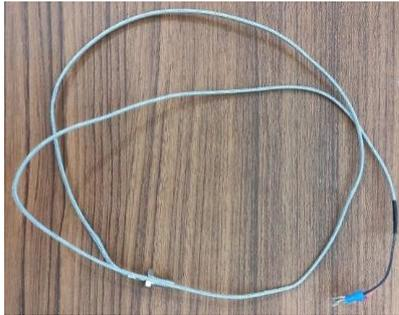
Gambar 3. 5 *Thermocouple*
