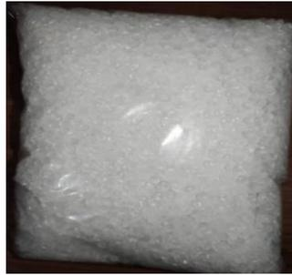
Gambar 3. 1 Biji Plastik *Polyethylene Terephthalate* ( PET )
