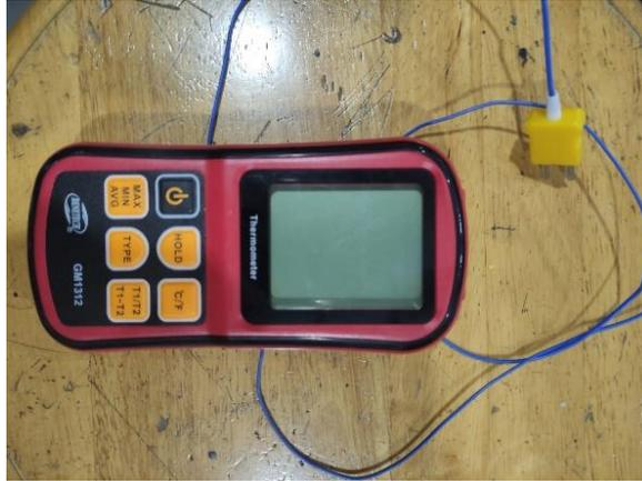
Gambar 3. 15 *Thermometer Digital tipe K*
